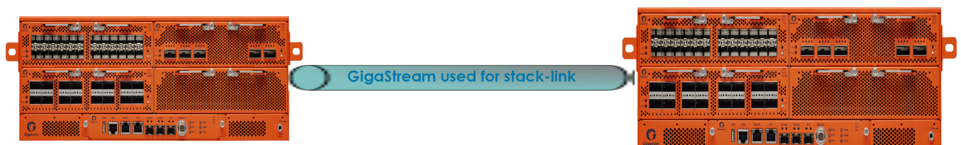
Figure 4 Daisy-Chain Configuration using GigaStream for Stack-link
